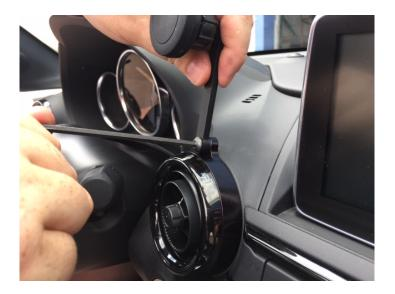
To install either phone holder, loosen the collar on the holder and pop the ball on the mount into the socket, then re-tighten the collar.
