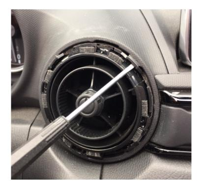
**<u>NOTE</u>**: It may be helpful to grasp the center of the vent and gently pull on the assembly as each of the four clips release.
