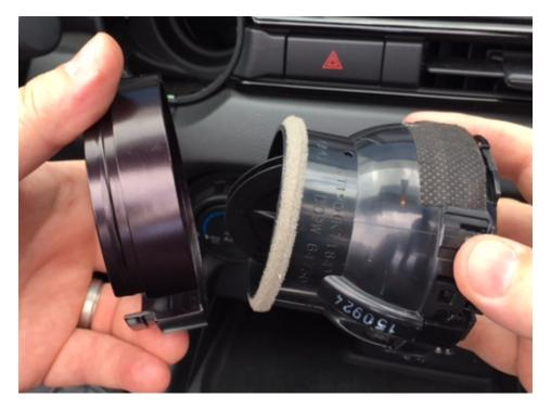
2. Press the two pieces together until the (4) clips of the vent assembly fully engage the groove inside the Vent Mount. You should be able to hear or sense the clips as they set into place.
