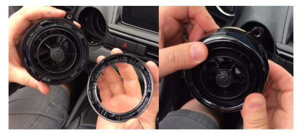
4. With the mounting tab on the Vent Mount oriented straight up, place the assembly back into the receptacle on the dash and with gentle but firm pressure, push the assembly into the dash until it fully seats.
