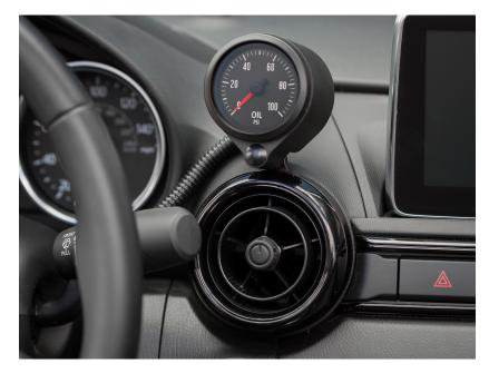
2. Install your gauge of choice and run the wires down alongside the gap in the adjustable steering column, into the dash, and down towards the fuse panel behind the drivers side kick panel. Finish your gauge install by following the instructions included with your particular brand of gauge.
