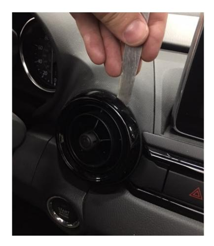
2. Once you have the trim ring popped off, use a small, flat-bladed screwdriver and release the vent assembly clips from the dash as follows:
