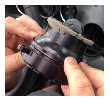
3. Set the vent trim bezel back onto the vent assembly making sure the (4) mounting clips are lined up properly and press together till the clips all fully engage.
