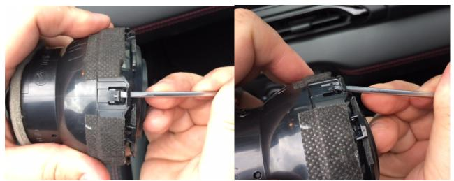
\*The above images show the required position of the screwdriver in relation to the clips.
