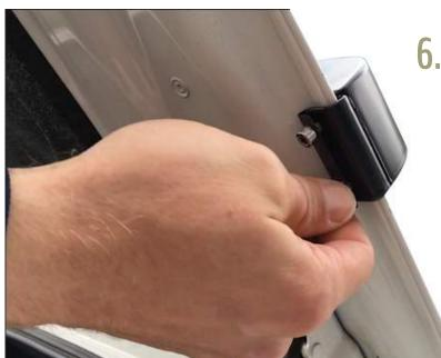
6. Use the supplied two screws on every bracket for extra fastening don't tighten these screws with to much force because than they can go through the protective 3-M strips
